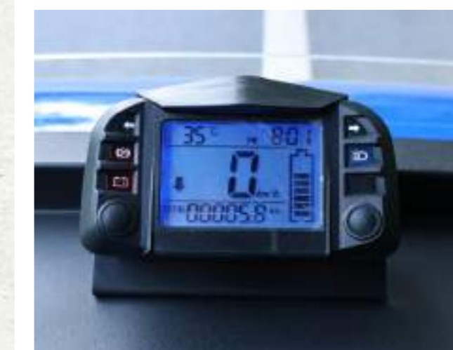
Speedometer integrated with speed display, mileage, battery indicator, temperature gauge, and clock
