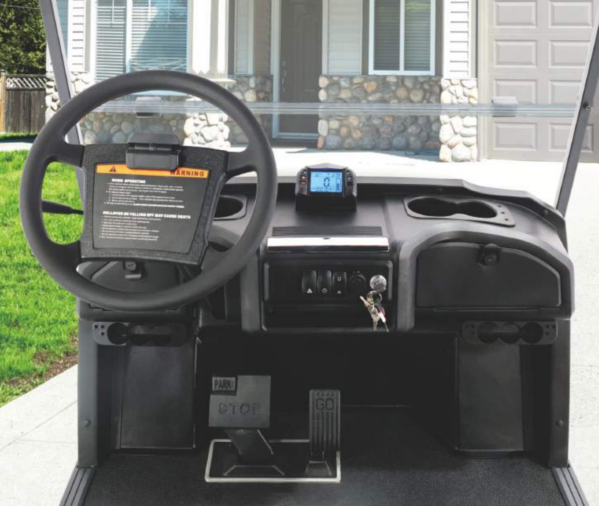
Speedometer integrated with speed display, mileage, battery indicator, temperature gauge, and clock
