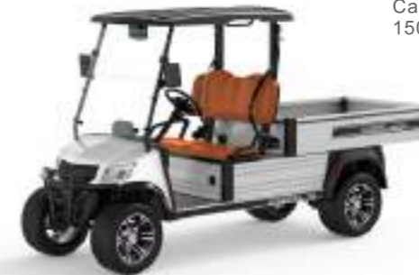
DU-CA500L-2 Cargo Bed Dimensions 1800 *1150 * 310mm
