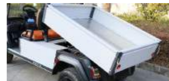
Aluminum rear cargo bed, loading capacity: 500 KGS
